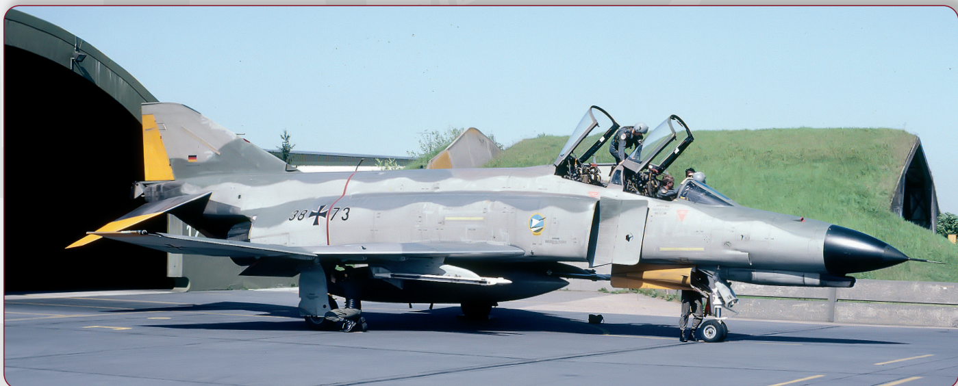
Style Variant 6: F-4F 38+73 of JG 74 "Mölders", seen in May 1992. Aircraft has Norm 81B camouflage, with wavy demarcation lines and hard edges, reaching higher-up on the fuselage sides. Of note is the small unit patch, which was introduced during the early 1990s.
