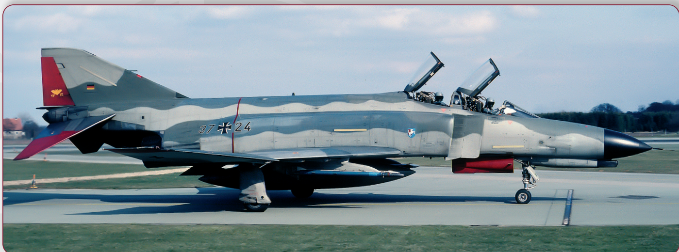
Style Variant 5: F-4F 37+24 of JG 72 "W", seen during the early 1990s, with Norm 81B camouflage, wavy demarcation lines and hard edges, reaching lower over the fuselage sides. The Phantom has red ID-colour on rudder, stabilizers, main landing gear door and wing tips. Most probably the stabilizers were painted red on the bottom surfaces as well. (Zetsche via AirDOC Collection)
