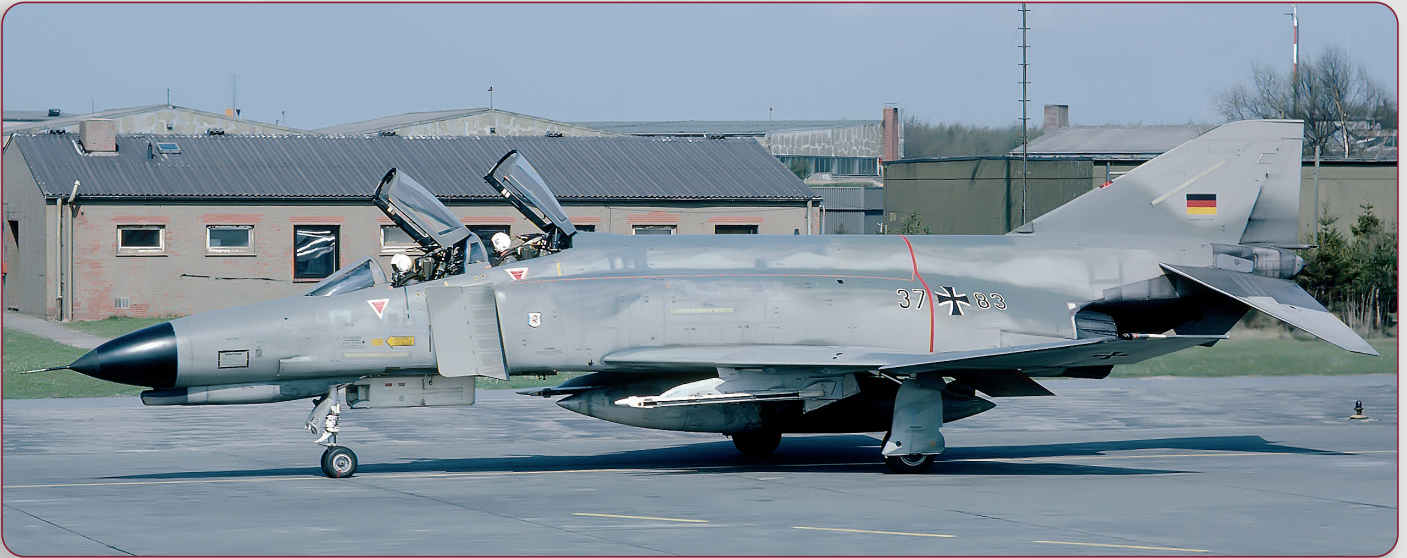
Style Variant 1: F-4F 37+83 of JG 71 "Richthofen", seen in 1984 at Wittmund, with Norm 81A "hybrid" camouflage (colour placement according to Norm 81A, but with more round Norm 81B-style lines). High demarcation lines on the fuselage sides and added, hand-sprayed soft contours. Large, early-style Iron Crosses on six positions and large German banner on fin. (Zetsche via AirDOC Collection)
